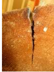
An example of radial splitting in wood.
